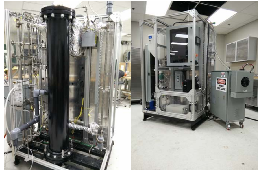
OHIO Prototype Internally-Heated SCW Reactor
